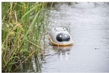
Length 0.6m, lightweight 7kg (excluding battery), no assembly required. Can be carried and used by one person.
