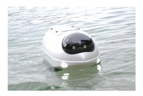
This new model has a function to return to the original position even after it is overturned in any water area. Two cameras (above and underwater) are mounted in this drone, and our default software is installed. This ensures that you can use our product very efficiently, meeting your specific use cases and requirements. The drone can be used for extended periods, allowing it to accomplish tasks on your behalf.
